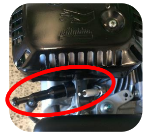
Disconnected spark plug
